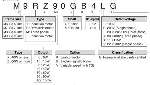
st Induction motor and reversible motor are single phase motor.
